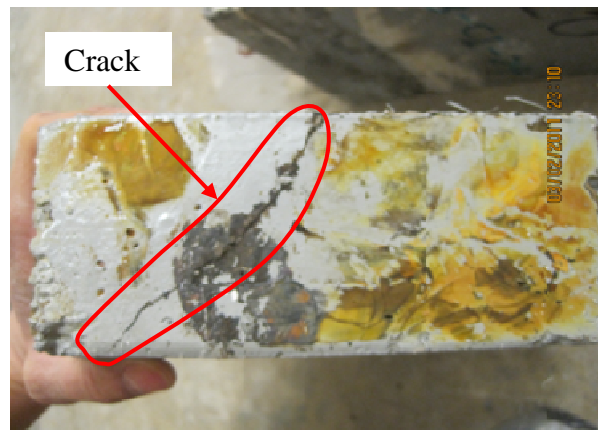
Figure 4.21. Cracks on specimen
