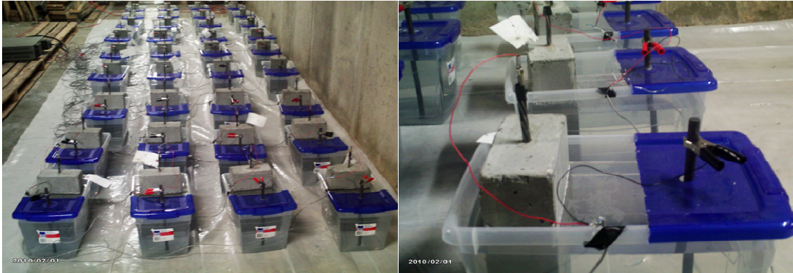
Figure 3.11. Accelerated corrosion test experimental setup
